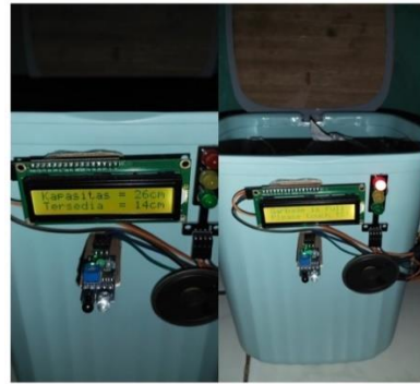
Figure 5. Ultrasonic sensor testing
